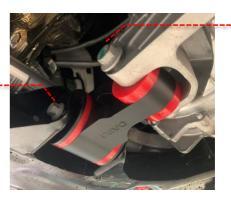
4 Finally torque the rear 16mm bolt to 47Nm and the front 16mm bolt to 45Nm. Reinstall the undertray. Reinstallation is the reverse of removal. Follow any factory torque specification during reinstallation of OE parts. Test drive the vehicle to ensure everything is okay. Your installation is now complete!
