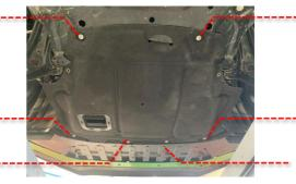
Remove the OE mount by first removing the rear 16mm bolt (A), then the 16mm front bolt (B). Once both bolts are out the mount should come out freely.
