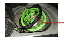
$38\,$  Refit the O-ring over the fuel lines and secure in place around the opening to the fuel tank.
