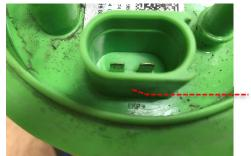
34 Inspect the fuel pump assembly lid to identify which wire is positive and which is negative that lead to the plug.
