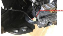
11 Remove the crash bar foam padding and place out of the work area
