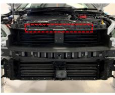
Push in the retaining clips on both sides of the upper radiator duct and remove the duct by lifting it up and away from the vehicle. Set the duct aside, out of the work area
