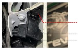
4 Disconnect the electrical connector and 2 wire routing clips shown
