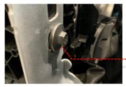
18 Remove the 1 x T30 screw from the radiator support clip, press the sides of the clip and slide it toward the engine. Repeat on the opposite side of the vehicle
