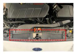
Using plastic trim tools, carefully pull the bumper cover sides outward to disconnect the cover from the chassis clips. Remove the bumper cover and set it aside, out of the work area
