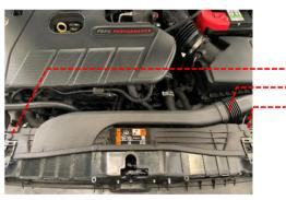
8 Disconnect the bonnet release cable and remove the cable from the routing clips as shown
