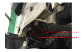
Tighten the 4 x 13mm bolts that hold the lower brackets to the Revo intercooler, then tighten the 4 x 13mm crash bar bolts, followed by the 4 x 10mm bolts holding the top brackets to the Revo intercooler and finally the 2 x T30 bolts holding the top brackets to the top radiator mounts.
