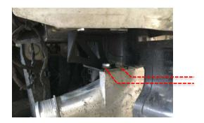
22 Refit the 4 x 13mm crash bar bolts, which now also go through the Revo lower intercooler brackets. Do not tighten yet. Remove the gearbox stand/hydraulic jack and square up the Revo intercooler.
