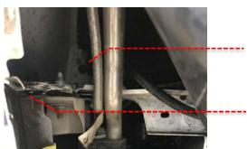
Remove  $5 \times T30$  and  $2 \times T25$  bolts that secure the front bumper to the main undertray.
