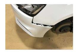
8 Whilst standing in front of the vehicle, carefully pull the bumper forwards to release it.
