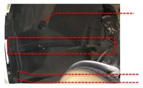
Remove the plastic push fit trim clip and the T30 bolt that holds the bumper to the wing. Repeat steps 1 and 2 on the opposite side of the vehicle.
