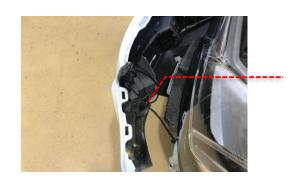
10 Remove the multiplug from the sensors at each end of the crash bar foam padding. Pull the red clip out and then squeeze the multiplug to release.
