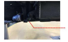
Position the Revo intercooler in front of the radiator and use a gearbox stand/hydraulic jack and a piece of wood to support it. Straighten the bottom radiator mounts and refit the 8mm bolts.
