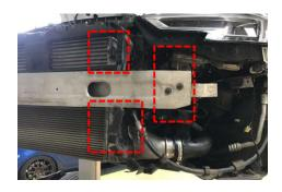
Refit all OE parts back to vehicle. Reinstallation is the reverse of removal. Follow any factory torque specification during reinstallation of OE parts. Check all sensors/electrics are reconnected. Also check bonnet release handle is refitted. Test drive the vehicle to ensure vehicle performs correctly and there are no leaks/part interference during operation. Your installation is now complete!
