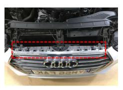
7 Carefully pull the bumper free from the corner at each side.
