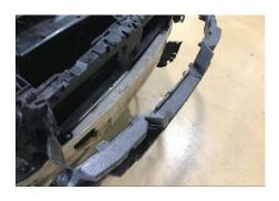
Remove the 2 x 13mm bolts and T30 bolt from each side of the crash bar and remove crash bar from the vehicle
