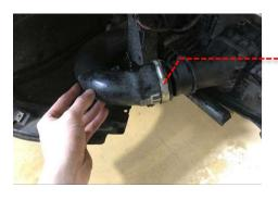
Using a pair of long nose pliers, release the clips at the top of the OE intercooler, one on each side.
