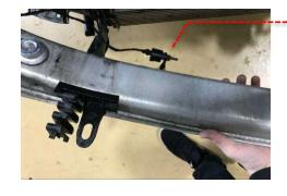
Using a 7mm socket, loosen the hose clip on the discharge pipe and remove the pipe from the OE intercooler. Repeat for the throttle pipe on the opposite side.
