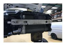
Fit the 2 x Revo smaller intercooler brackets to the top of the Revo intercooler using the 4 x 10mm bolts (supplied) and then refit the 2 x T30 bolts that go through the Revo bracket, crash bar and top radiator mount. Do not tighten yet.
