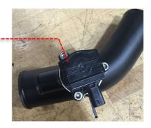
7 Using the OE discharge pipe as a guide, loosely assemble the Revo discharge pipe as shown using the two hoses, aluminium pipe and  $2\times60-80$  hose clamps.
