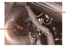
Install the new Revo throttle hose by inserting from the top of the engine bay and first connecting the hose to the throttle body with a 60-80 hose clamp, do not tighten yet. Next, under the car install onto the intercooler using a 60-80 hose clamp. Adjust the position of the pipes to get the alignment correct and tighten all the hose clamps, so the pipe is secure.
