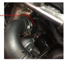
Remove the diverter valve from the OE discharge pipe and install on the new Revo discharge pipe using the 3 x M6x16 cap head bolts (supplied).
