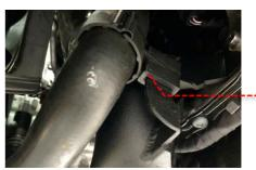
28 Install the remaining intercooler hose onto the Revo throttle hard pipe. Confirm that ~2-3mm of clearance remains between the hose and the underside of the air conditioning compressor after installation. Readjust the Revo throttle hard pipe if necessary to achieve a ~2-3mm gap between the hose and the air conditioning compressor. Once complete, tighten all throttle-side hose clamps (8mm socket).
