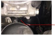
27 Install the coolant routing clip onto the Revo throttle hard pipe bracket.
