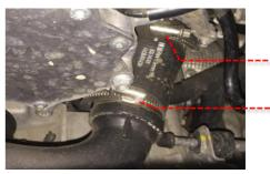
4 Loosen the mounting bolt on the discharge hard pipe (T30 bit).
