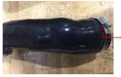
23 Install the Revo throttle hose into the engine bay, ensuring the Revo hose end with the internal step goes onto the throttle body. Rotate the hose on the throttle body until it has ~2.0mm of clearance to all parts within the engine bay. Install another provided 60-80mm hose clamp onto the open end of the hose.
