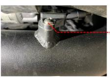
Install the Revo throttle hard pipe into the Revo throttle hose. Bolt the Revo throttle hard pipe to the block using the M6 x 20mm bolt (4mm hex bit) & M6 metal washer supplied, in the location shown. Place the rubber washer supplied between the Revo pipe bracket and block. Do not tighten the bolt yet.
