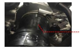
14 Remove the discharge hard pipe from the top of the engine bay and remove the coolant hose routing clip from the pipe (if installed). Set both aside, out of the work area.
