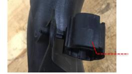
7 Loosen the hose clamp holding the stock hose to the throttle body (7mm socket).
