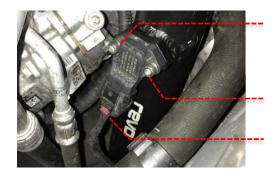
head bolts and washers (supplied). Reconnect the multiplug and push in the red tab to secure.
