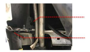
Remove the 5 x T30 and 2 x T25 bolts that secure the front bumper to the main undertray.
