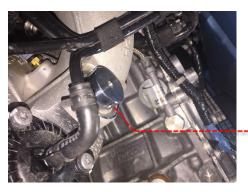
3 Install the Revo machined sound suppressor in the reverse of the removal of the OE unit, making sure you correctly refit the circlip.
