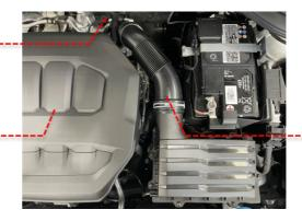
2 Remove turbo inlet pipe by loosening the T30 screw and then twisting back and pulling out of turbo.
