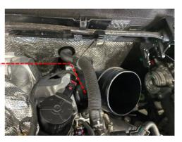
Remove the airbox lid by first pulling the breather hose off the side then loosen the 8 x T25 screws. Once open remove the OE filter and then using a flat head screwdriver pop the snow filter out of the base of the airbox, so you then have it as pictured.
