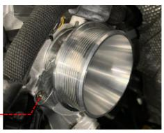
6 Install the new Revo inlet silicone hose with the supplied 70-90 hose clamps and tighten, re-install the engine cover. Your Installation is now complete!
