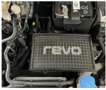
6 Install the new Revo intake silicone hose using the supplied 70-90 hose clamps. Click the DV pipe into the adapter and tighten hose clamps. Check everything is tight and your installation is complete.
