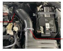
2 Remove the intake pipe from the car, unclipping the DV hose from the bottom of the pipe.
