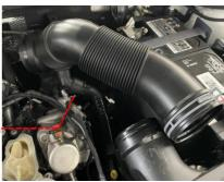
3 Loosely assemble the machined DV adapter using the 25-40 hose clamp onto the hose so you can twist it as required.
