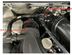
5 Remove turbo inlet pipe by loosening the 2 x T30 torx bolts holding it to the turbo.
