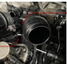
6 Vehicles with extra breather only - remove the take-off from the turbo inlet pipe using a pair of thin nose pliers to pop it out of housing.
