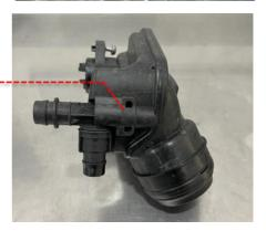
7 Vehicles with extra breather only - assemble the breather take-off pipe as shown using the silicone joiner pipe, machined joiner, machined take off adapter and hose clamps.
