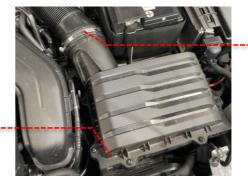
2 Remove both the air filter and large particle filter from the airhox
