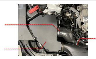
6 Finally apply your Revo badge to the top of the airbox as shown. Ensure all clamps and screws are tight and replace your engine cover.
