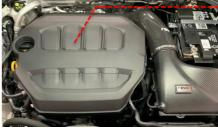
Remove the vacuum hose and secondary air injection hose (if equipped) from the airbox. Loosen the (8) airbox lid screws (T25 bit) and remove the airbox lid and intake hose. Remove the stock panel filter as well as the snow filter from the lower airbox -the lower airbox should appear as shown
