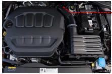
Loosen the stock turbocharger inlet bolt (T30 bit) and carefully move the inlet side-to-side to remove it from the turbocharger
