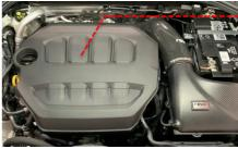
Loosen the clamp on the rear of the intake hose (7mm socket)
