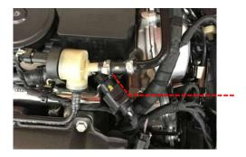
6 Loosen the hose clamp holding the breather hose onto the airbox lid and remove the hose.
