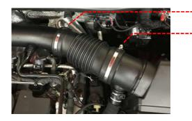
3 Loosen the hose clamp holding the intake pipe onto the turbo inlet.
