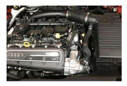
2 Loosen the 2 x hose clamps holding the rubber hose in place and remove from the vehicle.
