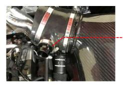
12 Attach the supplied vacuum line by pushing over the take-off. This does not need to be clamped.
