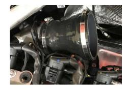
10 Attach the vacuum line (supplied) to the fitting on the Revo airbox coupler hose and secure with the hose clamp (supplied).
