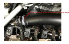
4 Remove the T30 bolt holding the intake pipe to the engine block.
