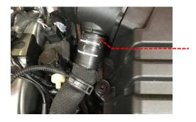
7 Using a T25, remove the 8 x bolts that secure the airbox lid and remove the lid from the vehicle.
