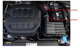
Remove the vacuum hose and secondary air injection hose (if equipped) from the airbox, gently pull up on the airbox to release it from the (3) engine bay grommets. Set it and the attached intake hose aside, out of the work area
