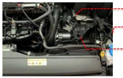
Unclip the coolant hose from the stock front section, remove the (2) front section screws (T25 bit), remove the stock front section and place it out of the work area
