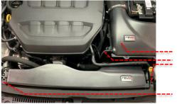
7 Reinstall the intake hose, start and test drive the vehicle to ensure there are no leaks/part interferences during operation. Your installation is now complete
